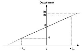
Notes: 1) The performance specified in the datasheet is valid within the 4-20 mA output range only 2) See arrow in the above diagram (dimensions).
